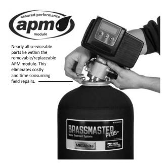
All BrassMaster and BrassMaster Plus water softeners / filters feature the Assured Performance Modular (APM) design. If you experience a failure of any valve component, the brass module can be easily removed and replaced with a factory remanufactured replacement module. Reference the BrassMaster and BrassMaster Plus Technical Video Library on our website (link is provided below) for detailed steps on how to remove the module. The required (downloadable) form to have your
