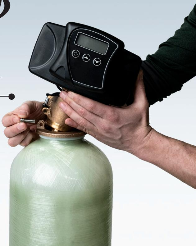
BrassMaster water softeners utilize the "ion exchange" process to remove undesirable hardness minerals. Incoming water passes through a bed of cation resin, where hardness is exchanged for very tiny amounts of sodium. Periodically, after a specified amount of hardness has been exchanged, a salt solution is used to "regenerate" the resin bed. Captured hardness minerals, along with excess salt solution, are sent to a drain. This leaves behind a recharged bed of resin, ready again for service.
