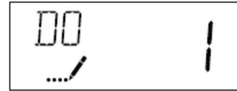
3. **Adjust Regeneration Time:** Press the Extra Cycle button to advance to next option. This setting determines the time of day that the unit will enter the regeneration cycle. The most common / default setting is 2:00 AM.
