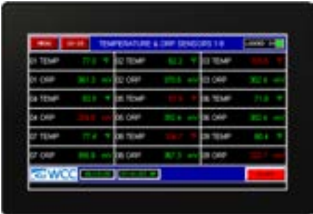
Example of ASHRAE 188 water temperature and quality monitoring via booster panel
